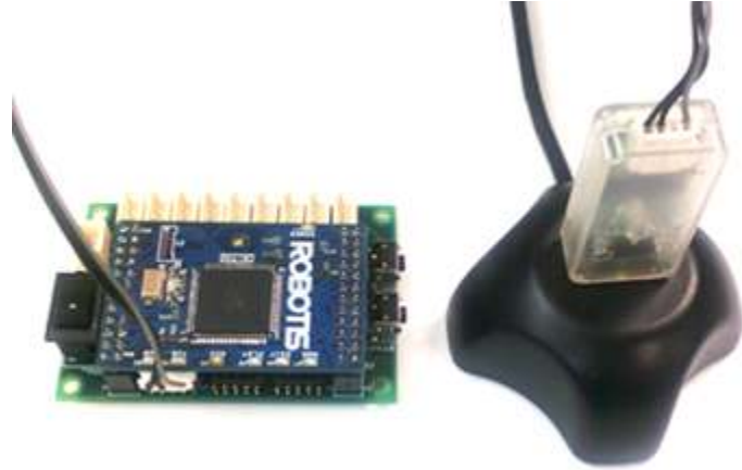
[The picture showing the connection of LN-101 and CM-700]
