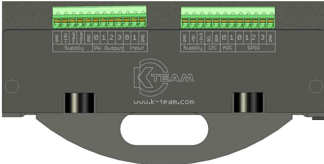
Figure 4.5: Terminal blocks connection
