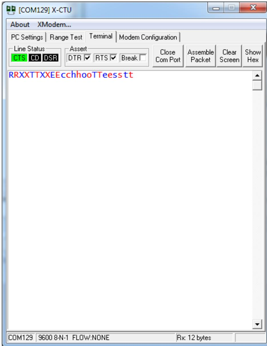
To do the DTR/DSR test, connect a wire from DSR to DTR line below
