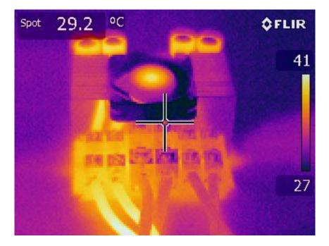
This thermal camera photo was taken with a Sabertooth 2x60 running 40A continuously on both motors. The left side is using 12ga stranded wire. The right side is using 8ga stranded wire. As you can see, the 12ga wire is not only heating itself up due to being undersized, but it is also causing heat to build up in the connections around it.
