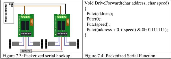
Example: So in this function, if address is 130, command is 0 (for driving forward), speed is 64, the checksum should calculate as follows:
