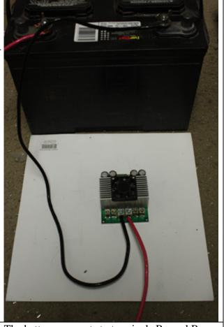
The battery connects to terminals B+ and B-
