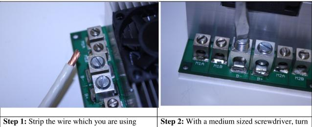
**Step 1:** Strip the wire which you are using approximately <sup>1</sup>/<sub>4</sub>". Use thicker wire for high current applications. *See the chart on the next page for wiring guidelines.*
