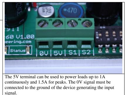
2x60. There is no need for an external BEC unless you need more than 1 Amp. The BEC will work at full rated output throughout the Sabertooth's operating voltage range. You can use the BEC at full capacity whether you are running 7V or 24V in.
