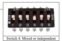
Sabertooth 2x60 is in Independent mode. In **Independent** mode, the signal fed to S1 directly controls Motor 1 (outputs M1A and M1B) and the signal fed to S2 controls Motor 2.
