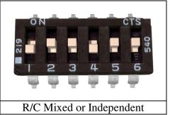
turning of the vehicle. When switch 4 is in the DOWN position, Independent mode is selected. In this mode, the signal fed to the S1 input directly controls Motor 1 (M1A and M1B) and the signal fed to S2 controls Motor 2.
