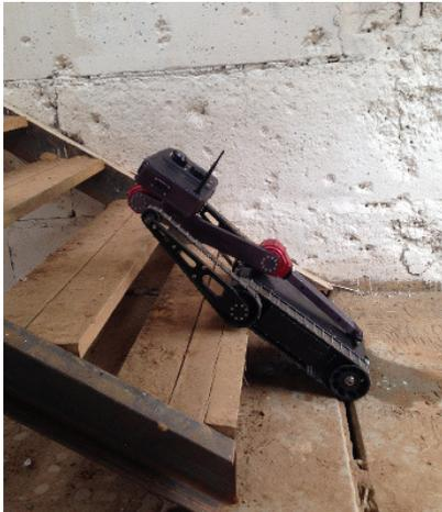
The small size of the robot enables it to easily traverse doorways and narrow passages either inside damaged buildings or outdoors while carrying a powerful array of sensors and tools.
