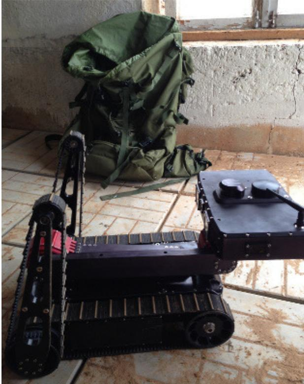
The robot is designed to have as small weight and footprint as possible while still meeting the requirements of being able to climb stairs and raise the sensor head high enough to look inside parked cars. The robot fits inside a regular backpack and can be simply carried to a mission area by its human operator. Backpack transportability is a required feature when it comes to using the robots in hard-to-access areas where transportation by cars or trucks is impossible.
