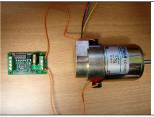
The motor connects to terminals M1 and M2
