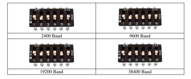
What baud rate to use is dependent on what your host can provide and the update speed necessary. 9600 baud or 19200 baud are recommended as the best starting points. If communication is unreliable, decrease the baud rate. If communications are reliable, you may increase the baud rate. The maximum update speed on the SyRen 50 is approximately 2000 commands per second. Sending characters faster than this will not cause problems, but it will not increase the responsiveness of the controller either.
