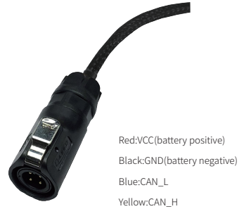
Figure 3.2 Schematic diagram of aviation plug male connector
