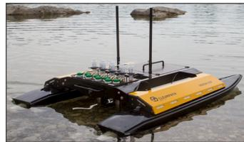
Heron is ideal for **bathymetric surveys and ecosystem assessment**. Load it up with sonar, magnetometers, water quality sensors and samplers. GPS telemetry is available to geo-locate data.
