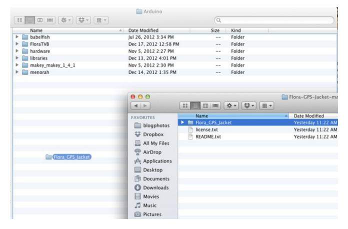
Unzip the package and drag the Flora\_GPS\_Jacket folder into your Arduino folder (located by default in Documents on OS X). Open the enclosed Flora\_GPS\_Jacket.ino file in the Adafruit Arduino IDE. (http://adafru.it/aVE)
