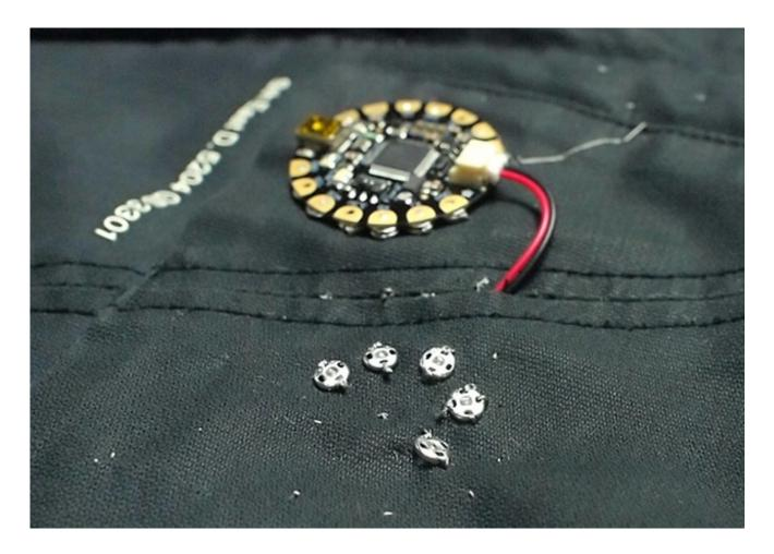
Attach the GPS next! You can sew it directly to your garment or make it snappy with our Flora with Snaps tutorial. Connect 3.3v on the Flora to 3.3v, GND to GND, and RX->TX and TX->RX.
