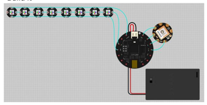
Here's a diagram of the jacket's circuit. You'll chain eight pixels together around the collar and attach the GPS to 3.3v, TX, RX, and ground. A 3xAAA battery holder hides in a pocket and extends through a seam to plug into the JST port on the Flora.
