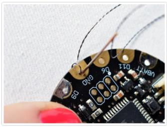
Make the connections in your circuit with conductive thread.
