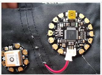
You can hide the conductive thread traces just under the top layer of fabric, just make sure the stitches aren't so long that they can move and come into contact with each other. You can see that the thread periodically appears on the outside of the garment to anchor the stitched lines.
