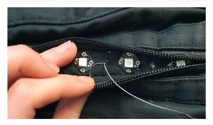
Then connect up the short data connections between each pixel. Be sure to seal the knots with clear nail polish or Fray Check.
