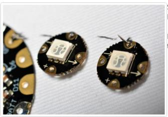
Start by stitching the ground bus from GND on Flora to the (-) pads on each pixel.
