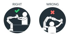
DO NOT place your head or other body parts between or underneath segments of the robotic arm!
