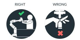
NEVER place body parts (especially hands, fingers) between the robotic arm or its end effector and stationary objects.
