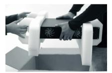
Work in twos to remove the foam packaging of the Control, one person holding the Control and the other removing the foam packaging.
