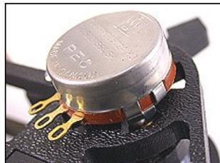
9. Slide the potentiometer through the plate opposing the bearing hole. Before passing through the bearing on the opposing side, install the lockwasher, jam nut, and the upright that was assembled in step 7. Tighten the jam nut to secure the potentiometer but **do not** tighten the clamping hub.
