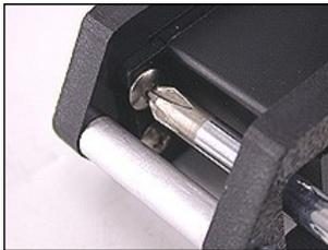
17. Fasten the servo to the frame with the (4) #4 x 1/4" black truss head phillips screws. **Do not tighten screws so that you can adjust the gear mesh in the next step.**
