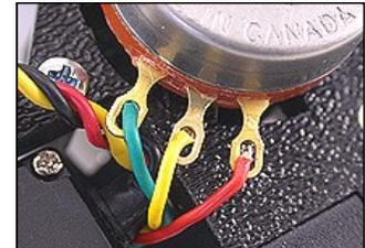
20. Remove the stock potentiometer on your modified servo and solder the potentiometer wires to the external potentiometer in the following order:
