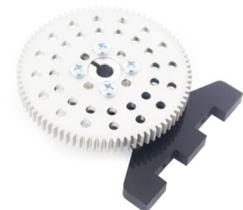
12. Attach the spur gear to the hub on the remaining upright (assembled in step 8) with 6-32 x 1/4" pan head screws. Note that the cupped portion of the gear faces toward the upright.
