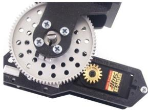
18. Insert the pinion gear onto the servo and re-install servo screw. Slide the servo toward the hub gear to achieve a snug (but not tight) gear mesh and tighten the servo mounting screws.
