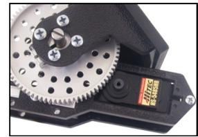
16. Place the servo in the frame as shown.
