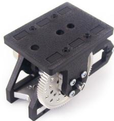
14. Attach the top plate as shown using the (4) #4 x 1/2" flathead screws. This is a tight fit and may need to be tapped on with a hammer.
