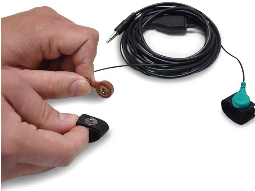
Figure : GSR connecting GSR electrodes
