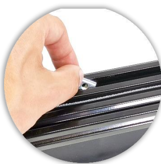
Put a blocker in the rail where you want the sensor to be
