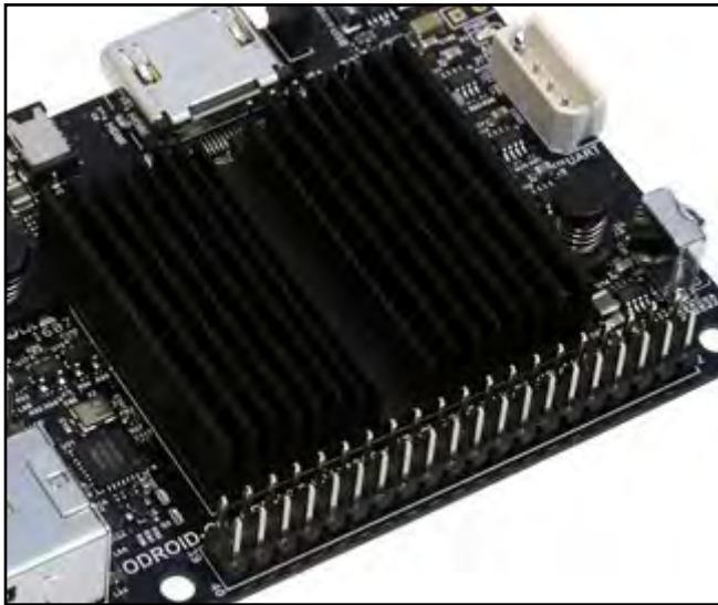
Heatsink attached to the ODROID-C2
