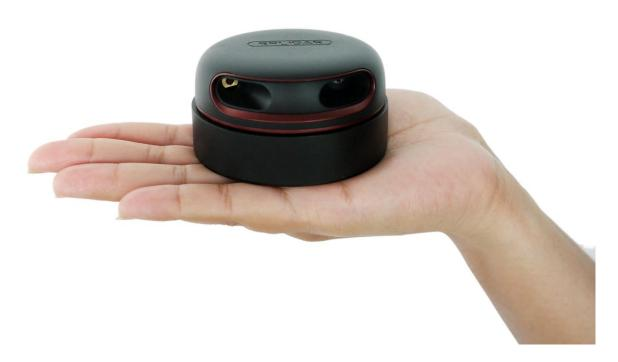
The RPLIDAR A2 is the next generation low cost 360 degree 2D laser scanner (LIDAR) solution developed by SLAMTEC. It can take up to 4000 samples of laser ranging per second with high rotation speed. And equipped with SLAMTEC patented OPTMAG technology, it breakouts the life limitation of traditional LIDAR system so as to work stably for a long time.
